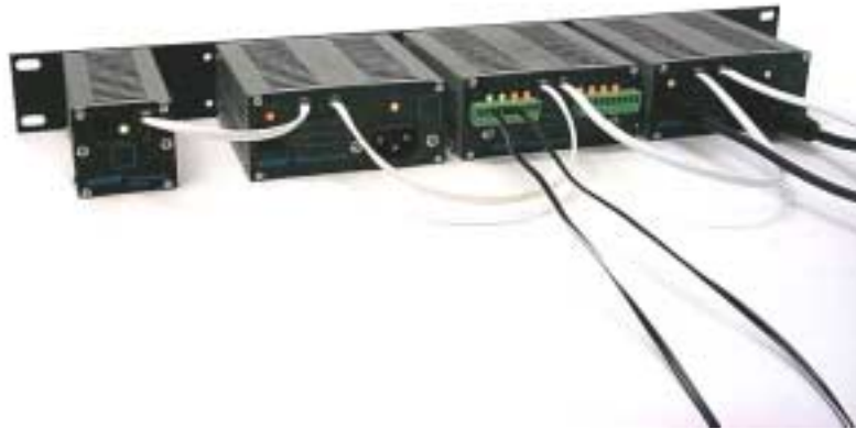
Figure 4: MARS sensors mounted on RP8 rack panel
