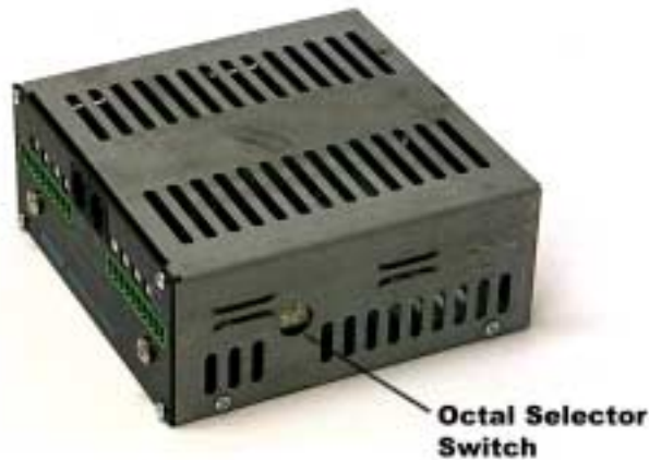
Figure 7: Sensor module depicting address selector
