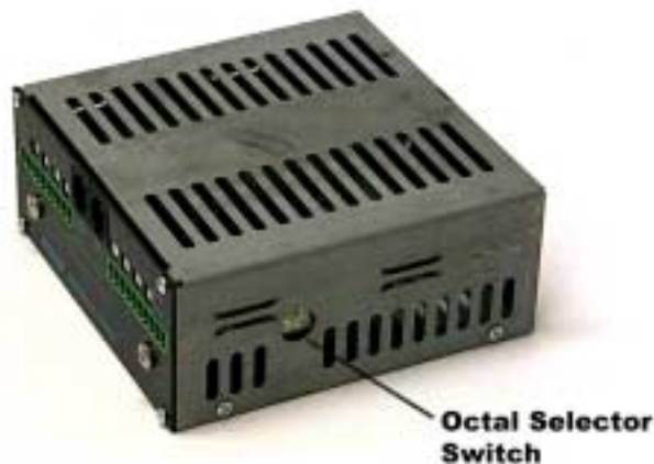
Figure 7: Sensor module showing address selector
