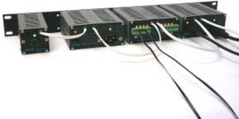
Figure 1: MARS sensors mounted on RP8 rack panel
