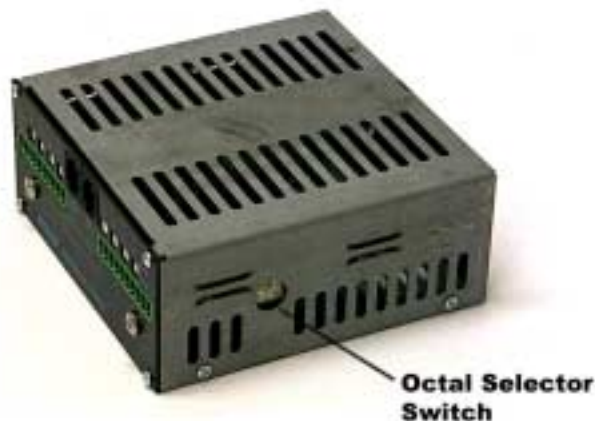
Figure 6: Sensor module showing address selector
